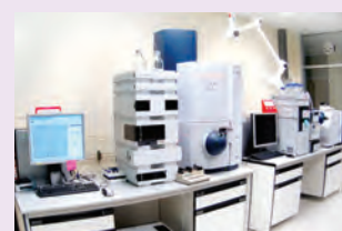
Analysis of drugs and metabolites using LC/MS (TOF) and LC/MS/MS (Ion Trap).
