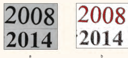
Figure 5: Images of printed characters and Xerox characters. (a) visible light image; (b) classified image displayed in "false" colour.
