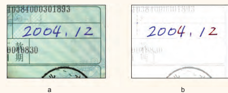
Figure 4: Altered bank check. (a) visible light image; (b) classified image displayed in "false" colour.
